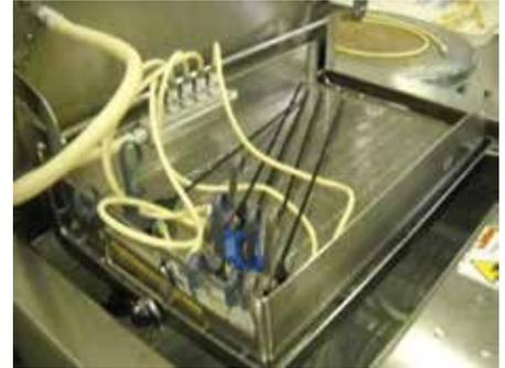
Figure 2: Irrigating instruments
