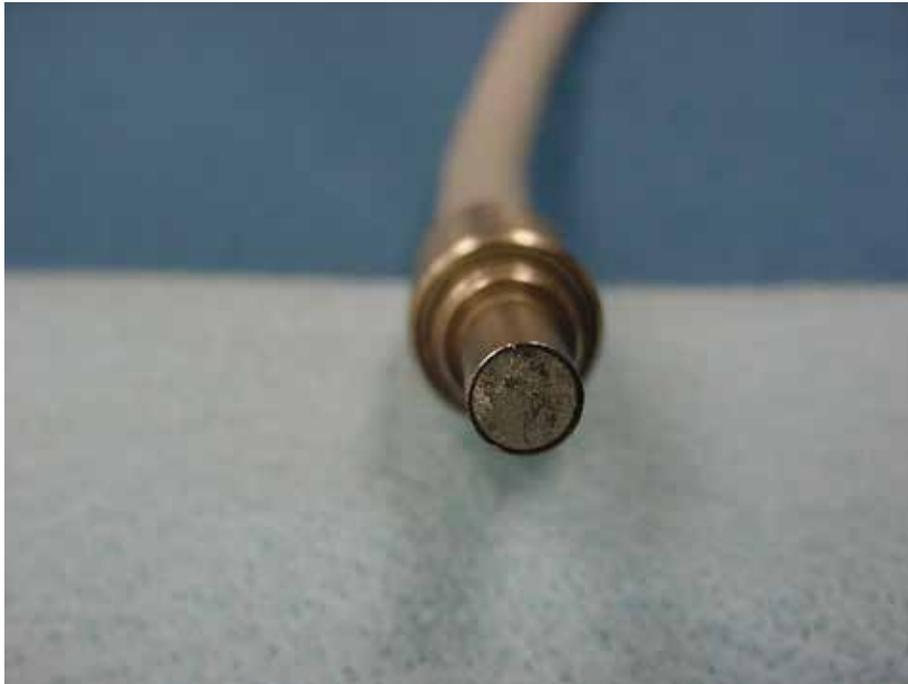
Figure 4: A light cable with broken fibers
