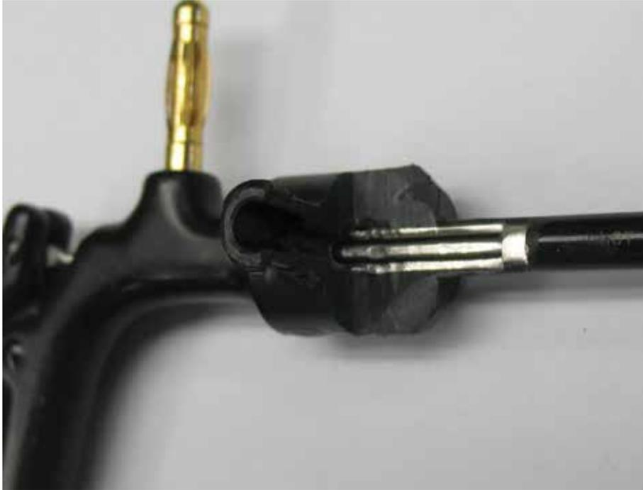
Figure 1: Dissected flushing port shows the intersection with the instrument shaft
