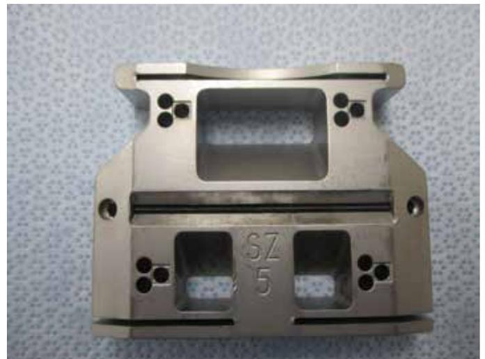
Figure 5: Cutting Block
