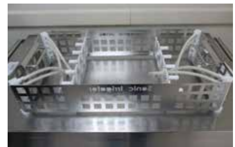
Figure 7: Robotic instrument accessory for an ultrasonic cleaner
