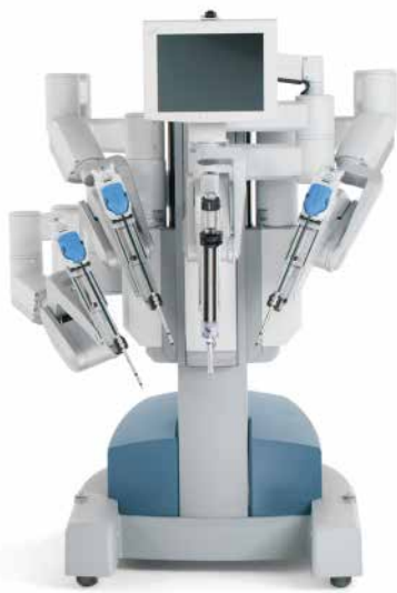
Figure 3: Robotic patient cart with instruments and telescope in place
