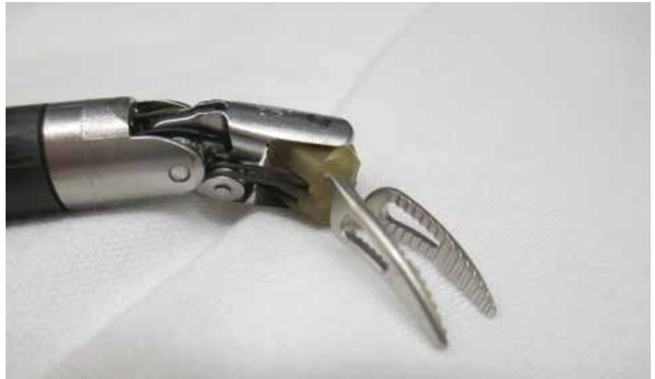
Figure 4: Distal tip of a robotic instrument showing exposed cables
