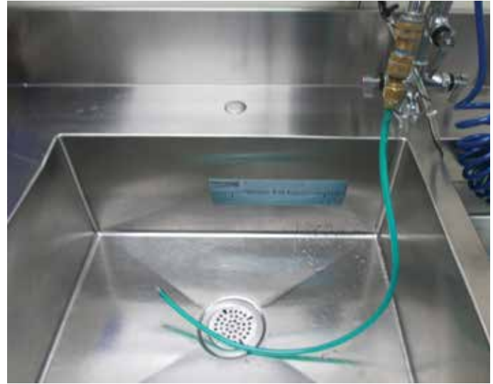
Figure 6: Pressure-specific hose for flushing the ports of a robotic instrument
