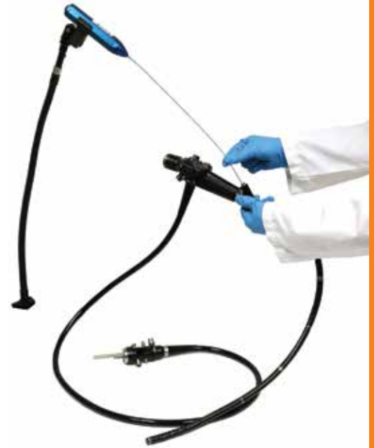
Figure 8: Example of a Flexible Video Borescope for Internal Inspection of Endoscope Channels
