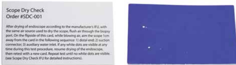
Figure 7: Example of an Endoscope Drying Test – Side 1 is instructions, Side 2 is for detection. White dots on blue/purple background indicate moisture is detected.
